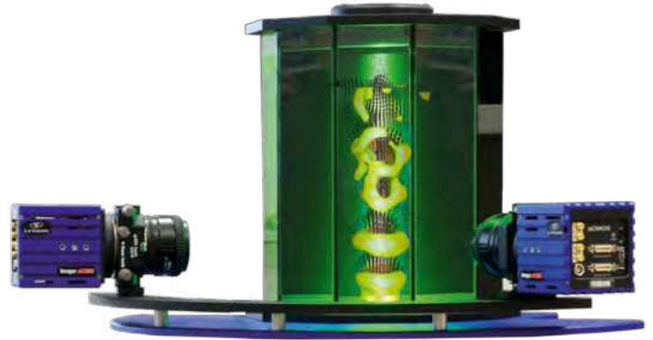
2-camera Tomo-PIV setup
