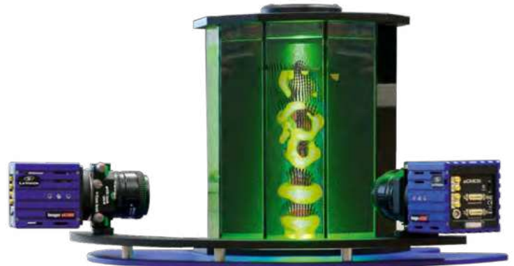
3D flow field of a liquid jet (page 7)
