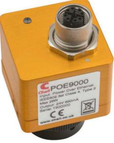
The Chell Power Over Ethernet (PoE) adapter can be fitted onto any of the TE NetScanner range and brings the convenience of PoE to these products.
