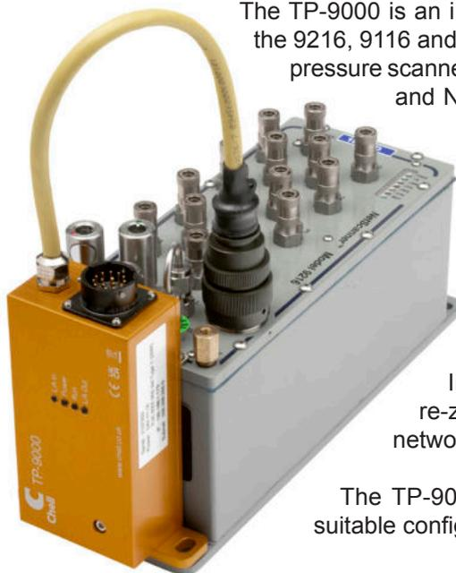
The TP-9000 is an iDDS and Power-Over-Ethernet (PoE) interface for the 9216, 9116 and 9016 pressure scanners. It effectively brings these pressure scanners up to the latest interface standards. The TP-9000 and NetScanner brick can be powered either by PoE or 24 VDC. The TP-9000 will automatically configure itself for the power supply that is available.
